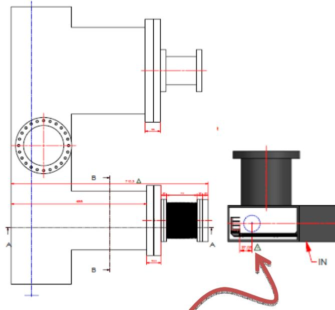
coincident  $^{15}\text{O}$  or  $^{19}\text{Ne}$  detected at  $\sim 1^\circ$  with 6 pin diodes in UHV
