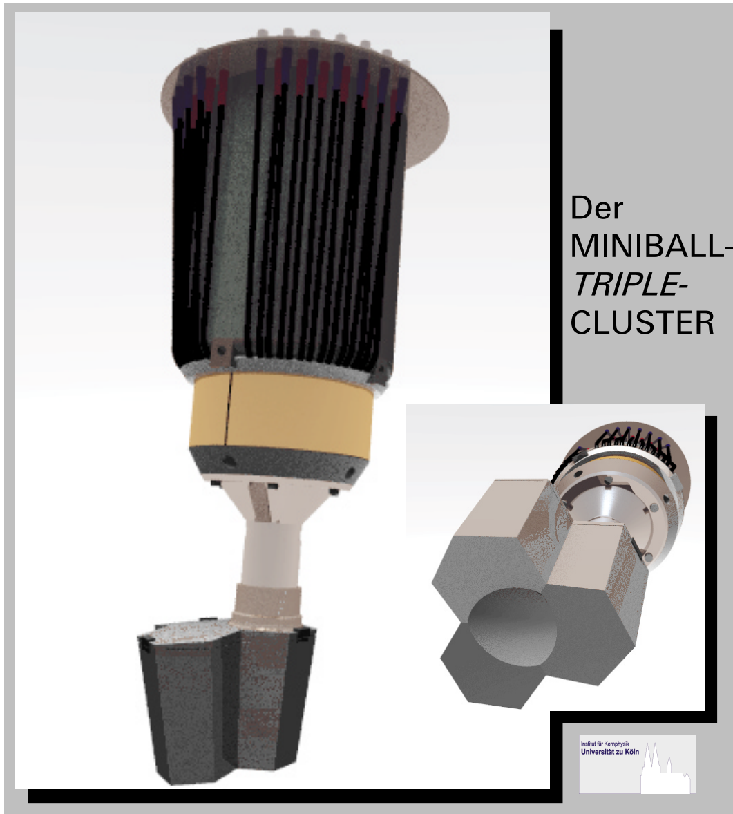
Figure 2.4: The new MINIBALL 3-Cluster cryostat (asymmetric solution). (Courtesy of Universität zu Köln)
