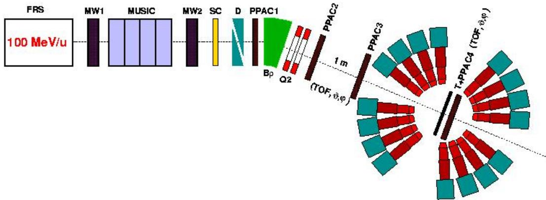
**Fig. 3:** Schematic drawing of the experimental set-up for slowed down beams.
