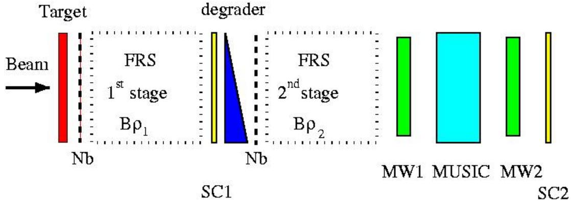
**Fig.1:** Schematic drawing of the projectile fragment separator with the standard detector set-up for in-flight identification of ions prior to the secondary target.
