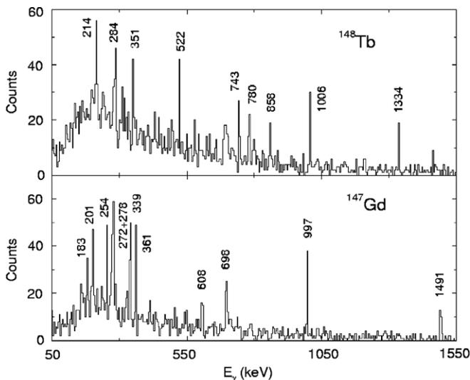
Fig. 3.  $\gamma$ -Ray spectra associated with the decays of the high-spin isomers in  $^{147}\text{Gd}$  [11] and  $^{148}\text{Tb}$  [12] as observed following the projectile of the  $^{208}\text{Pb}$  beam. These decays represent the highest discrete spins observed to date in projectile fragmentation reactions.
