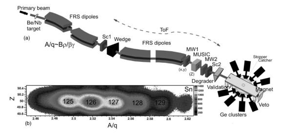
FIG. 1. (a) Experimental setup and (b) the identified Sn isotopes from <sup>238</sup>U fission.
