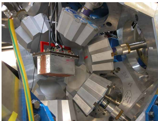
Fig. 3. Photograph of the DSSSDs in-situ at the centre of the RISING array in its Stopped Beam configuration. The active stopper is housed in the light tight box in the middle of the opened array.
