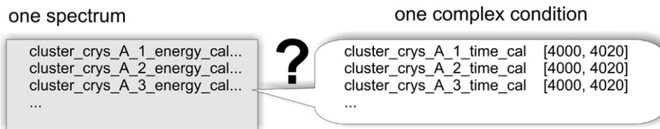
Fig. 15. A very common error, usually made by beginners during defining a conditional sum spectrum. It is not enough to create just one condition and depending of its current logical value, increment the spectrum (or not). The proper solution is shown on the next figure.
