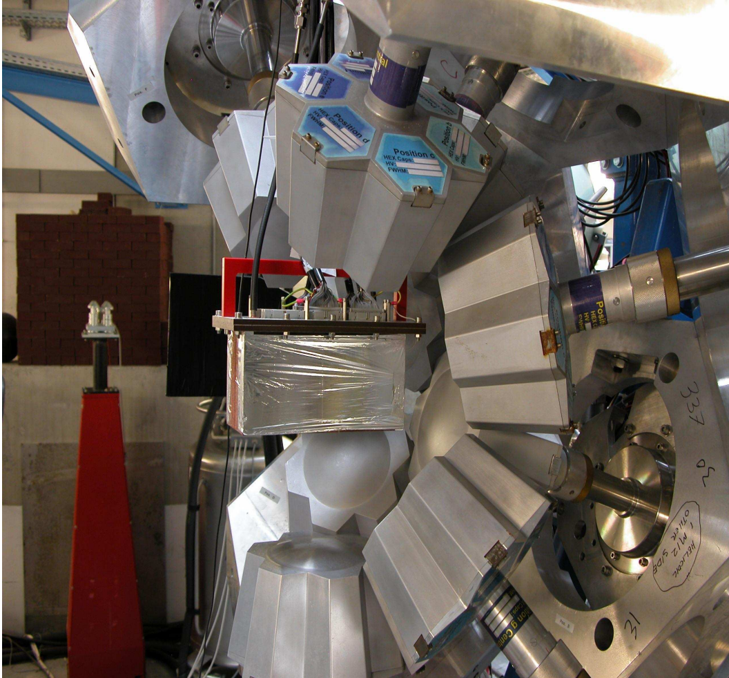
Figure 3.14: A photograph of the active stopper surrounded by the RISING germanium clusters.
