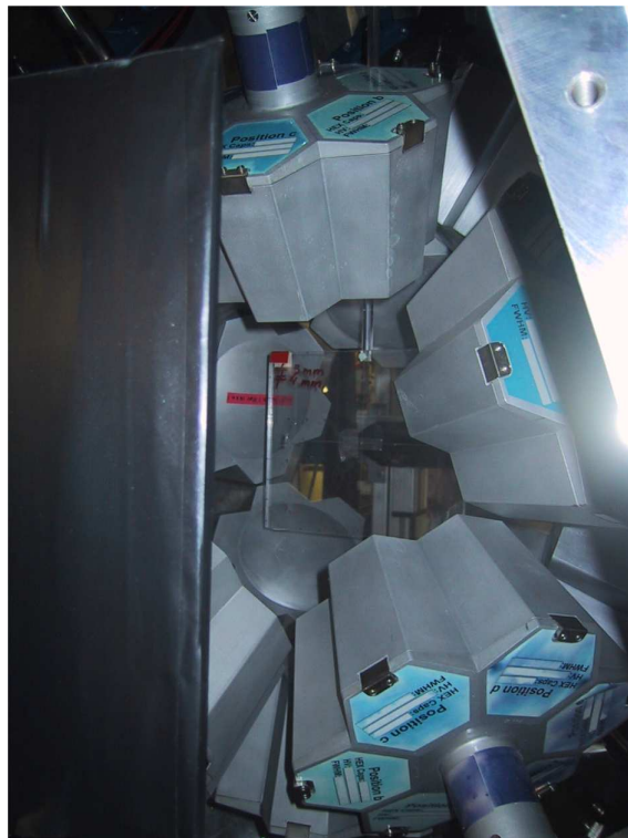
Figure 3.11: Photograph of the Stopped RISING array with the 7 mm perspex stopper mounted in the centre. In the foreground can be seen the veto detector, scintillator 43 (black object to the left).
