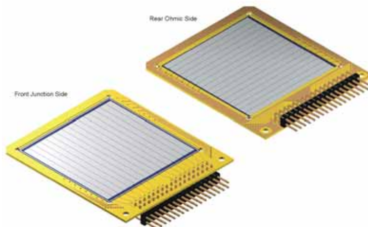
Fig 2: Schematic drawing of the W1(DS)-1000 double-sided silicon strip detector (DSSSD) from Micron Semiconductor Ltd. [1].
