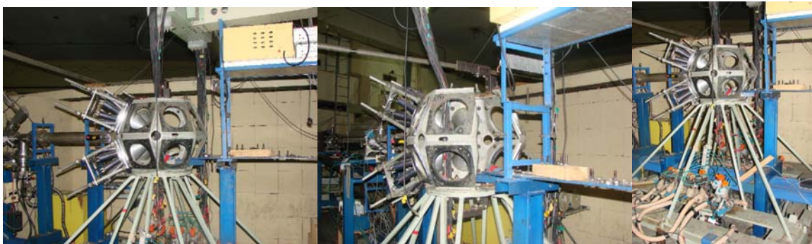
Fig.2 shows the experimental setup with the annular parallel plate avalanche counter (PPAC) and two Ge-detectors at backward angles. The optimal setup will include four Clover Ge-detectors at backward angles ( 153^{\circ} ). The azimuthal angles are 25^{\circ} , 155^{\circ} , 335^{\circ} and 205^{\circ} . The front face radius of the Clover detector is r=3.25(6) cm. The intrinsic photopeak efficiency for the Clover detector is \epsilon=0.20 . The increase of the intrinsic photopeak efficiency from \epsilon=0.13 , the value for the individual Clover diodes, corresponds to the add-back factor.
