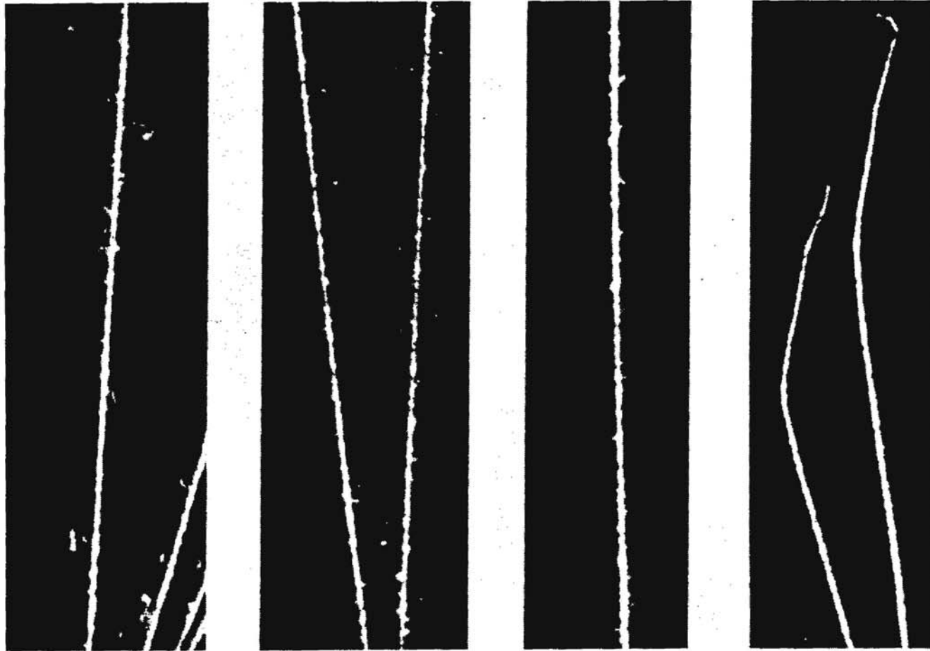
Figure 2-4 Cloud-chamber tracks of alpha rays showing delta rays. The first picture is in air, the last three in helium; the gas pressure in the chamber is such that the tracks cross about 10^{-5} g cm -2 of air equivalent. Note nuclear collisions in the section on the right. [T. Alper, Z. Physik , 67, 172 (1932).]
