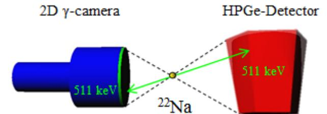
Advantage over conventional scanner: Full detector can be scanned in one measurement
