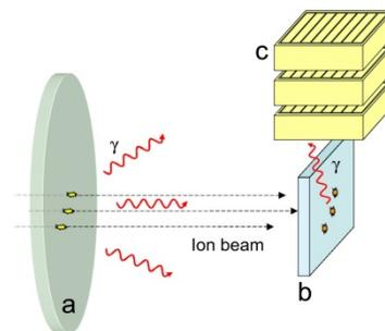
*Background suppression* and P/T can be improved by applying imaging techniques.
