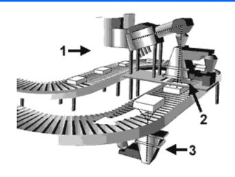
'Cold pasteurization' or 'electronic pasteurization' uses electrons (from an accelerator) or X-rays produced using an accelerator.
