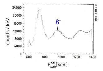
Delayed sum-energy spectrum taken at 590 MeV. (delayed time window 20-65ns with respect to beam pulse) A peak associated to the  $K^\pi\!\!=\!\!8^{\text{-}}\!\!$  shows up. The other peaks correspond to isomers of fusion products from target contaminants
