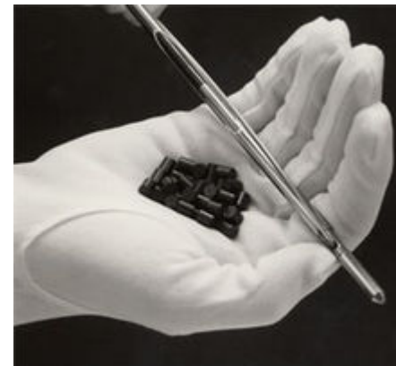
A fuel rod and Uranium-oxide pellets, the fuel of most power reactors.
