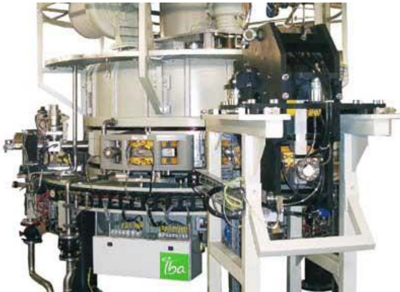
The IBA rhodotron – a commercial accelerator used for e-beam sterilization
