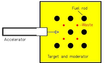
A subcritical reactor with additional neutrons produced by 1 GeV protons.
