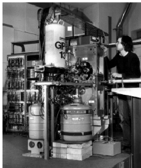
TESSA2 6 Compton suppressed Ge detectors
